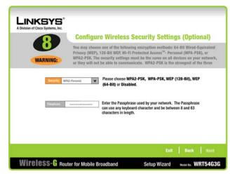
Figure 5-11: Configure Wireless Security Settings - WPA2-PSK Screen
